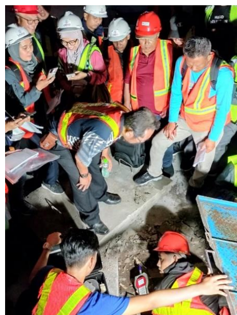
Participants are measuring minimum night flow using an Ultrasonic Flow Meter (UFM) at Perum Korpri.
